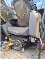
Image Comment(s):Seat not inflatting/rising - 2 pin plug for compressor locking tab missing
