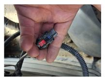
Image Comment(s):Seat not inflatting/rising - 2 pin plug for compressor locking tab missing
